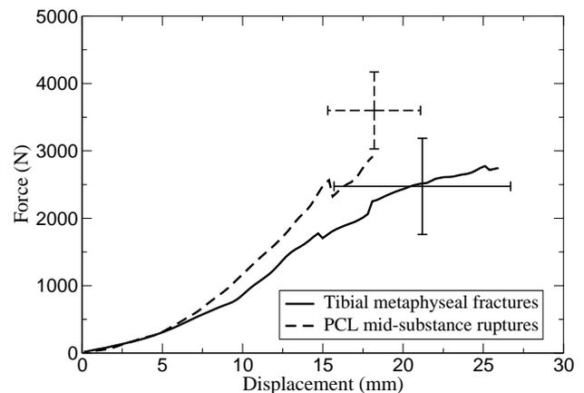
**Figure 2:** Average force-displacement responses for tibial metaphyseal fractures (n=7) and PCL mid-substance ruptures (n=4).
