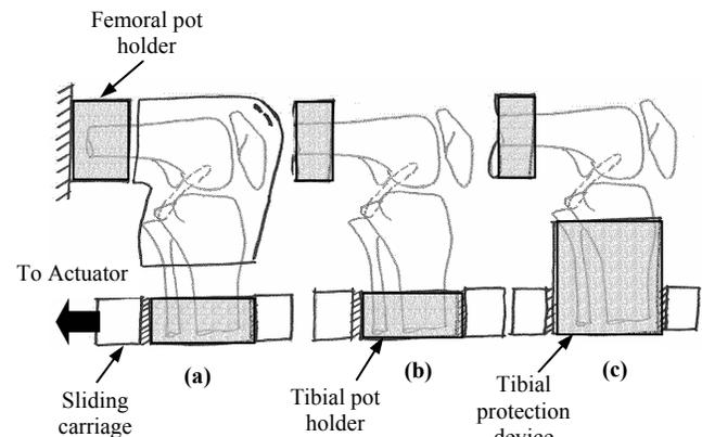
**Figure 1:** A schematic diagram of (a) Intact knee-Series I (b) PCL only knee-Series II (c) PCL-only knee with tibial protection device-Series III.
