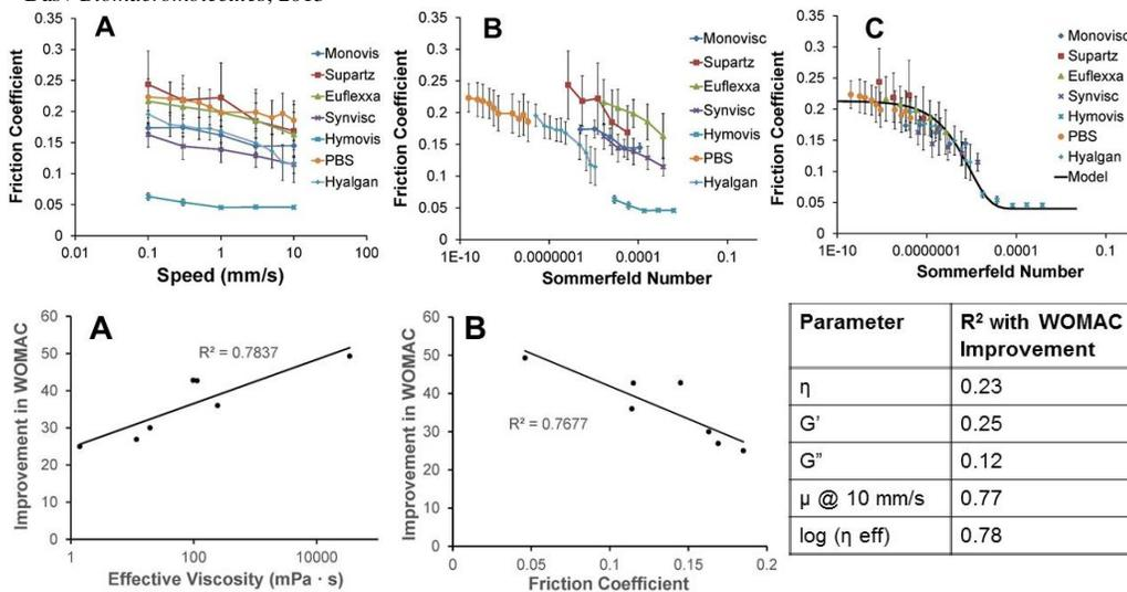
**Figure 1:** Comparison of friction coefficients for HA products as a function of speed (A) and Sommerfeld number (B) using measured viscosities. Fitting data to elastoviscous transition curve for a model lubricant enabled calculation of effective lubricating viscosities that collapsed all data sets onto a single curve. (n = 4)
