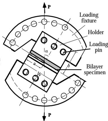
Figure 1. Mixed Mode Sandwich specimen
