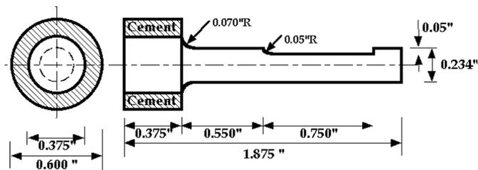
Figure 1. Test Specimen.
