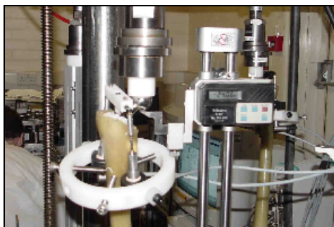
Fig 1 - Measuring the prosthesis head migration with height callipers. Circular frame used to mount the LVDT's.
