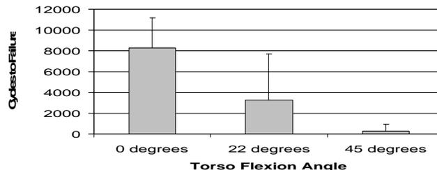
Figure 1. Average cycles to failure of lumbar motion segments at different torso flexion angles.
