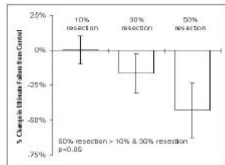
Figure 3: Load bearing capacity for differing amounts of resection.
