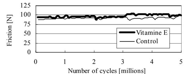
Figure 3. Frictional force measured during simulator testing.
