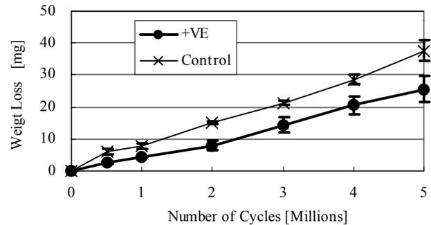
Figure 2. Weight loss due to wear on the knee joint simulator.
