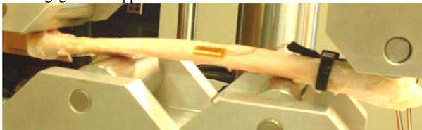
**Figure 2: Image of canine radius in four-point bending apparatus.**
