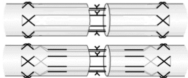
Figure 1. Top – Simplified 6-strand locking repair. Bottom - Modified Savage repair. Image modified from Viinikainen 2004<sup>5</sup>
