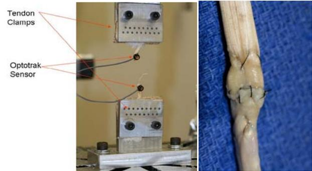
Figure 2. Left - Tendon specimen in custom tendon clamps mounted to servo-hydraulic testing machine after test. Right - Flexor tendon repaired with the simplified locking technique and epitendonous stitch, using multifilament stainless steel suture and 5-0 Nylon respectively.
