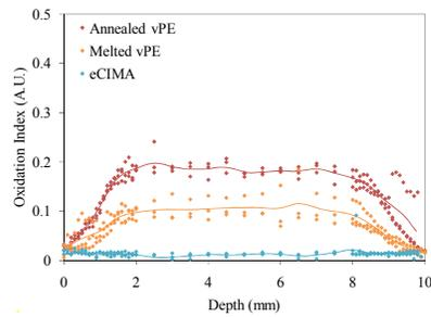
**Fig 1:** Oxidation profiles after ASTM F2003 aging. Actual data from all samples in a group is represented by the individual data points; the splined average of the three profiles in each sample group is shown as the solid line.
