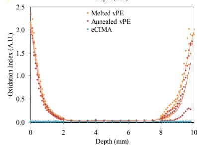
**Fig 2:** Oxidation profiles after squalene doping and pressure vessel aging. Actual data from all samples in a group is represented by the individual data points; the splined average of the three profiles in each sample group is shown as the solid line.
