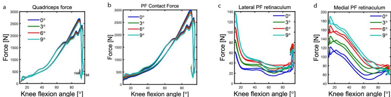
Figure 3. Quadriceps muscle forces (a), patellofemoral contact forces (b), lateral (c) and medial (d) patellofemoral ligament forces.
