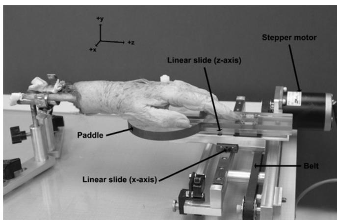
Figure 1. The cadaveric wrist mounted on the custom made motion simulator which is controlled by a laptop.
