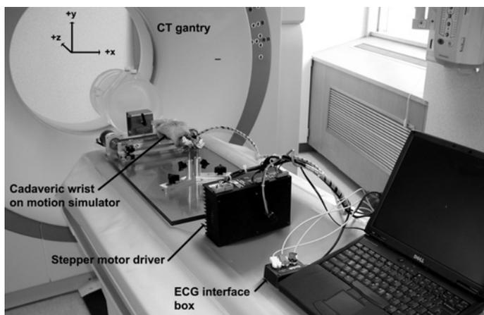
Figure 2. The setup used for 4D CT scanning.
