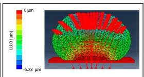
Fig.2 Cross-sectional view of Z-displacement in ABAQUS. FE model displaced 5.23  $\mu m$  to reach the measured target nuclear height of 9.9  $\mu m$ .
