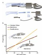
Fig. 1. A) Model of assembled device. Clear parts are biological bone. Blue metal parts are for modeling purposes only. Titanium metal parts make up physical device. C) MCP vs. IP angles for biological thumb vs. device. IP angle extrusion point indicated by arrow.
