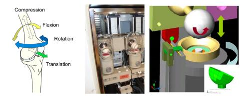
Figure 1. Articular motion is a combination of complex multiaxial load (Left). This can be mimicked using a ceramic hip ball bioreactor system (middle) that is able to recapitulate the articulating motion (right).
