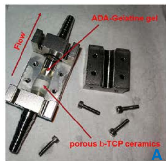
Fig. 1: Flow chamber with \beta -TCP and ADA-gel (A); released DAP and BMP-2 concentrations (B); cumulative release curves for DAP and BMP-2 (C)
