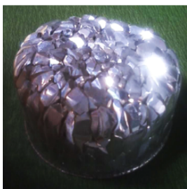
Figure 1. Magnesium after refining
