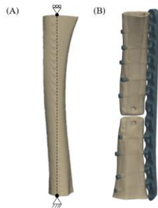
Fig. 1: Representative models for intact control limbs and operated limbs with constraints. (A) Simplified loading conditions were defined using a pinned support on distal end and roller support on the proximal end. (B) A 12-hole stainless-steel plate and screws were virtually implanted in the operated limb models.
