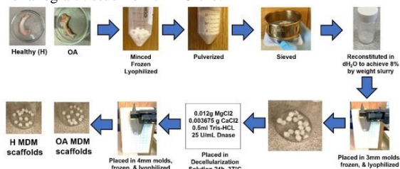
Fig 1. Fabrication procedure of H and OA MDM scaffolds.
