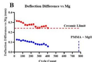
Figure 2. A) Results of dynamic deflection with non-linear fitting. B) Dynamic deflection differences per cycle using MgO cement as the baseline.
