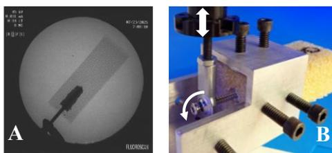
Figure 1. Dynamic testing post 48 hour curing time. A) All cement types infused within the open foam osteoporotic bone blocks. B) Cyclic testing of bone blocks with swivel rod end to maintain axial loading during screw deflection.
