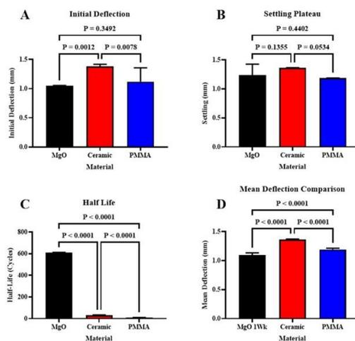
Figure 3. Dynamic testing post 48 hour curing time. A) Initial deflection, Yo. B) Settling deflection, Plateau. C) Half-life for stability. D) Mean dynamic deflection.
